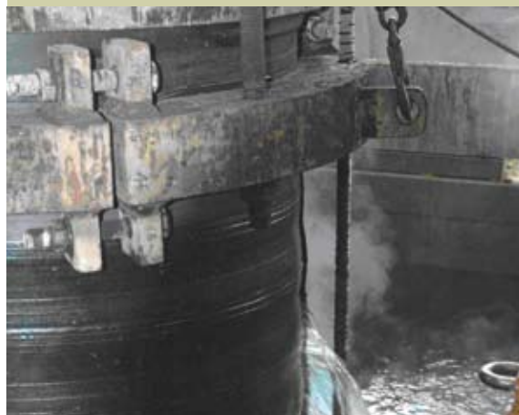
Burstpressure test of a KPPS pipe DN/ID 900 by 80°C
