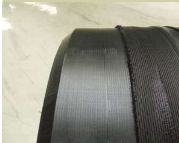
Electro fusion spigot of a DN/ID 1200 - 10 bar
